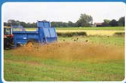
LOWLANDER 106 with 2 horizontal beaters and spinning discs, spreading poultry manure
