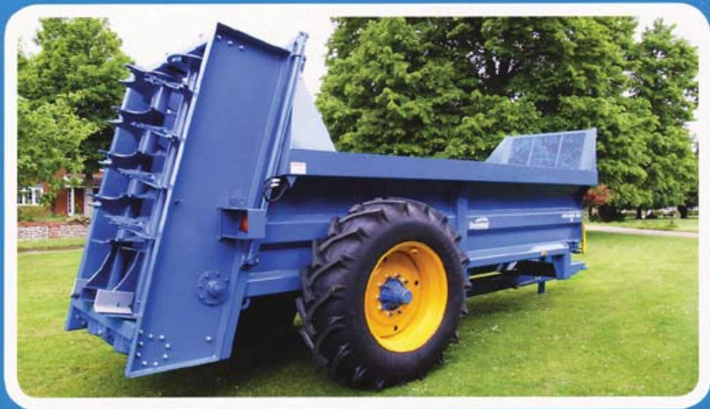
LOWLANDER 90 with high augers and gullotine slurry door
