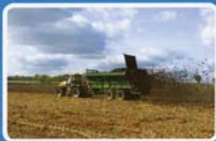
230 WIDEBODY sludge cake build with built in flared extension sides and guillotine slurry door
