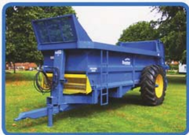
LOWLANDER HD 150 with gliotline slurry door and sprung drawbar.
