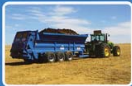
350 WIDEBODY with 2 horizontal beaters and spinning discs, 530mm bolt on extension sides, 2 steering axles, guillotine slurry door and sprung drawbar
