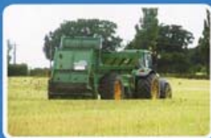
160 WIDEBODY with 2 horizontal beaters and spinning discs, load cells and 710/70 R38 tyres
