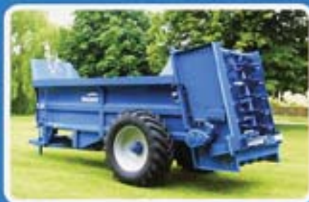
LOWLANDER HD 150 sludge cake build with guillotine slurry door
