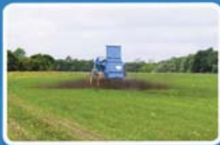
LOWLANDER 150 with 2 horizontal beaters and spinning discs, weigh cells, bolt in flared extension sides, gullotine slurry door and sprung drawbar
