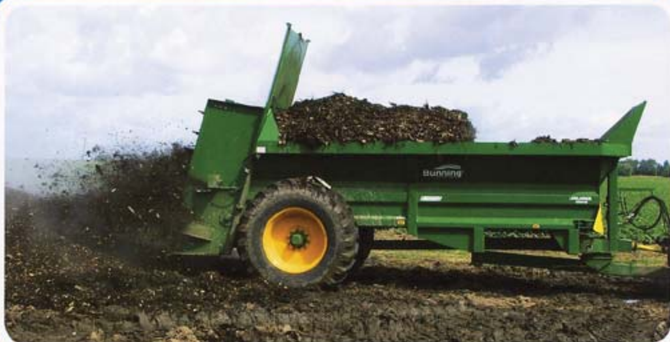
LOWLANDER HD 150 sludge cake build with flared body, guillotine slurry door, 710/70 R38 tyres and load cells, composting
