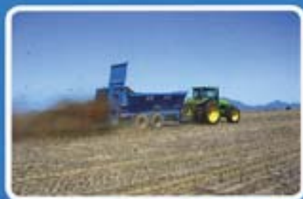
230 WIDEBODY with 530mm bolt on extension sides and guillotine slurry door
