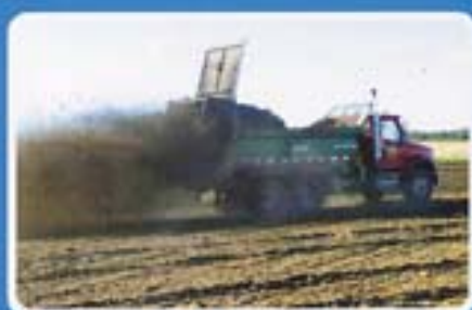
140 WIDEBODY TRUCK MOUNT with guillotine slurry door
