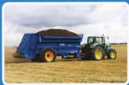
LOWLANDER 150 with detachable spinner deck, weigh cells, bolt on extension sides, gullotine slurry door and sprung drawbar
