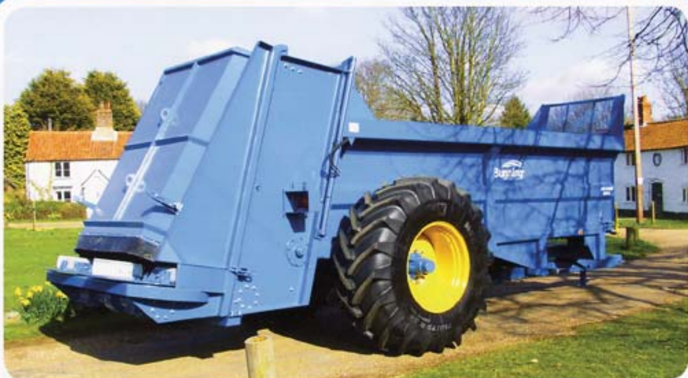
LOWLANDER HD 150 with detachable spinner deck, guillotine slurry door and sprung drawbar
